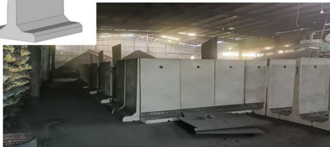
Concrete Wall ( T Shape)
